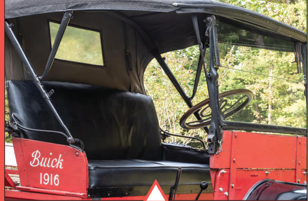
The D-4 Express was repainted just once in its factory-spec red, with the Buick script and model year added at some point, perhaps for parade duty. The folding top was optional, and it appears to wear a later foldable windshield.
