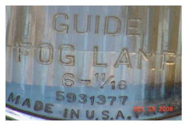
Lens detail for 6-11/16 inch. This is the same detail for two color or single color lens. Both lens types have the same cast-in part number.
