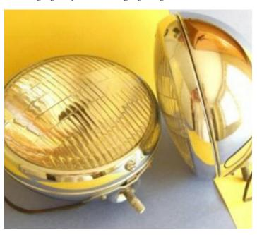
Guide 6-11/16" Light. ID is mounted at the top center on the back shell.
