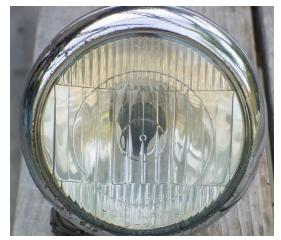
The Guide round (Guide part number unknown) 5-3/4" light was designed for the 1941 Oldsmobile and has a unique circular pattern on the lens (this light is shown in 1941 Oldsmobile literature).
