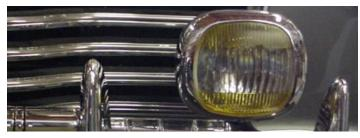
Close-up view showing light mounting. Note position closer to center obtained by reversing the Guide mounting brackets from that specified in the Buick Service Bulletin.
