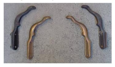
The Buick part numbers for the brackets were 5932053 Left and 5932054 Right. The cast iron brackets were painted semi-gloss black. The clamps were cadmium plated.
