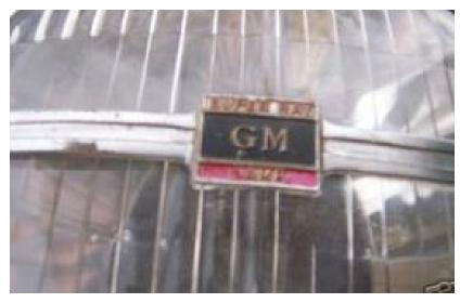
Note hood at top of bezel and horizontal badge and bar as contrasted with the vertical bar and shield of the prior generations.
