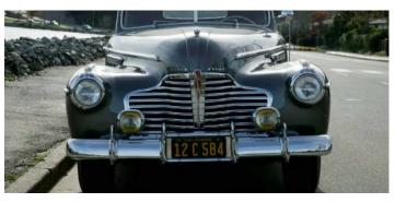
1941 Buick 71C in the Bulgari Collection (former Newton Cope car and referenced in Restoration Facts, 1941 Buick by William C. Anderson) with Guide 859-C lights and bi-color lens.
